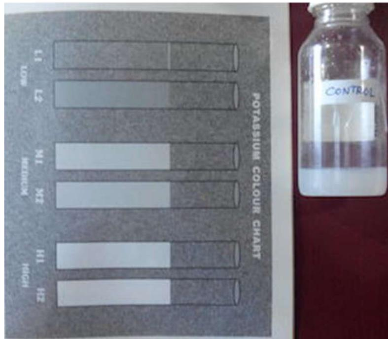
Figure 8: Indetermination of potassium content of soil in control, the color range falls in M2 for sample
